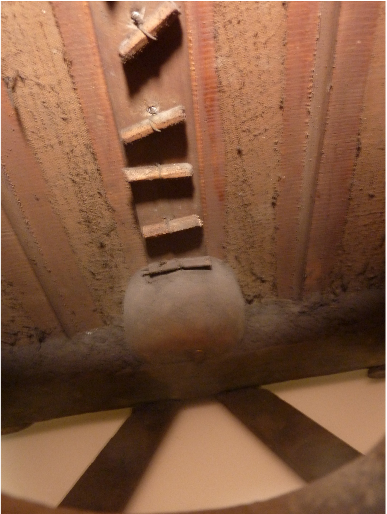
View through the lower rear access hole showing the front rail and the pillar attachment block. The tip of the pillar bolt is visible at the back of the block. You can also just see the backs of the front feet.
